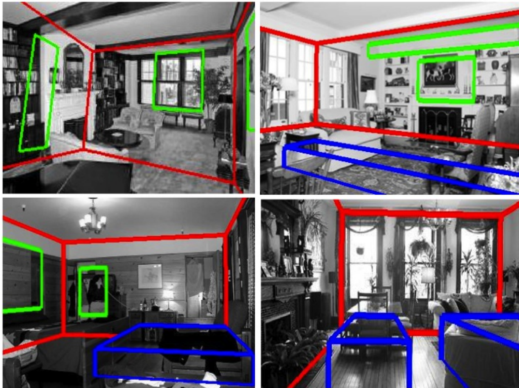
Figure 2.16: Some typical failures. Top left: The algorithm could not recover from a large error in the initial camera estimate. Top right: We often propose objects with unrealistic size, since there is no component in the model constraining object parameters to plausible values. Bottom row: our likelihood function is edge based, and objects that explain image edges very well might not correspond to actual pieces of furniture in the room. In the bottom left image, the contour of the predicted blue box is matched to edges generated by multiple objects in the image (the bed and the armchair).
