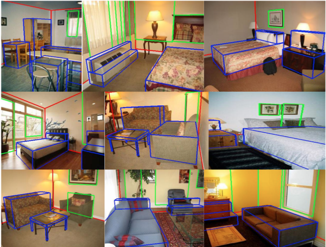
Figure 4.10: Some typical failures. Here, we show several cases where our method confused objects of different categories. For example, the table in the top left was confused with a cabinet, and the nightstand on the top right was wrongly labeled as a couch.
