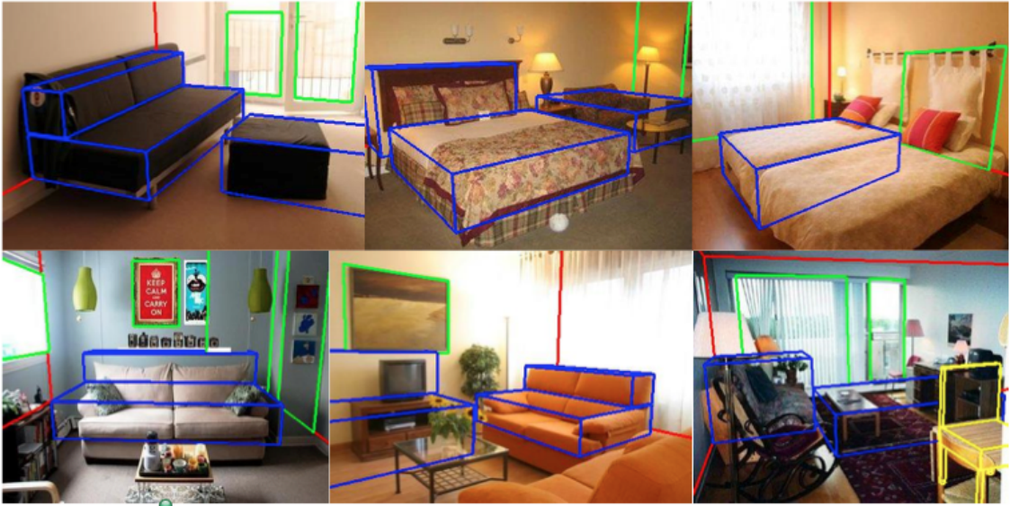
Figure 4.13: Failures in estimating the room box. Small mistakes in positioning the floor greatly affect object estimation. For example, positioning the floor too far behind results in having a cabinet behind the bed as opposed to a bed with a headboard (top middle), or poor couch estimates (top left, bottom left and middle). Sometimes the walls are not positioned correctly (bottom right).
