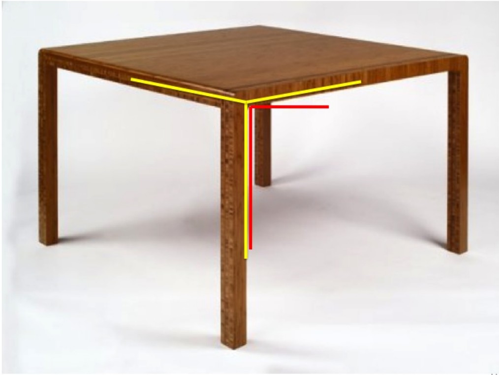
Figure 1.2: A perspective camera does not preserve angles. Here, the projected corner of a table (in yellow), which is orthogonal in 3D, is not a right angle on the image plane (compare it to the right angle denoted by the red lines). Notice how the four 2D angles corresponding to the table corners are all different. For this and other similar reasons, we model objects in the world using a three-dimensional representation, where shape and size have less variance than their projection in the image.
