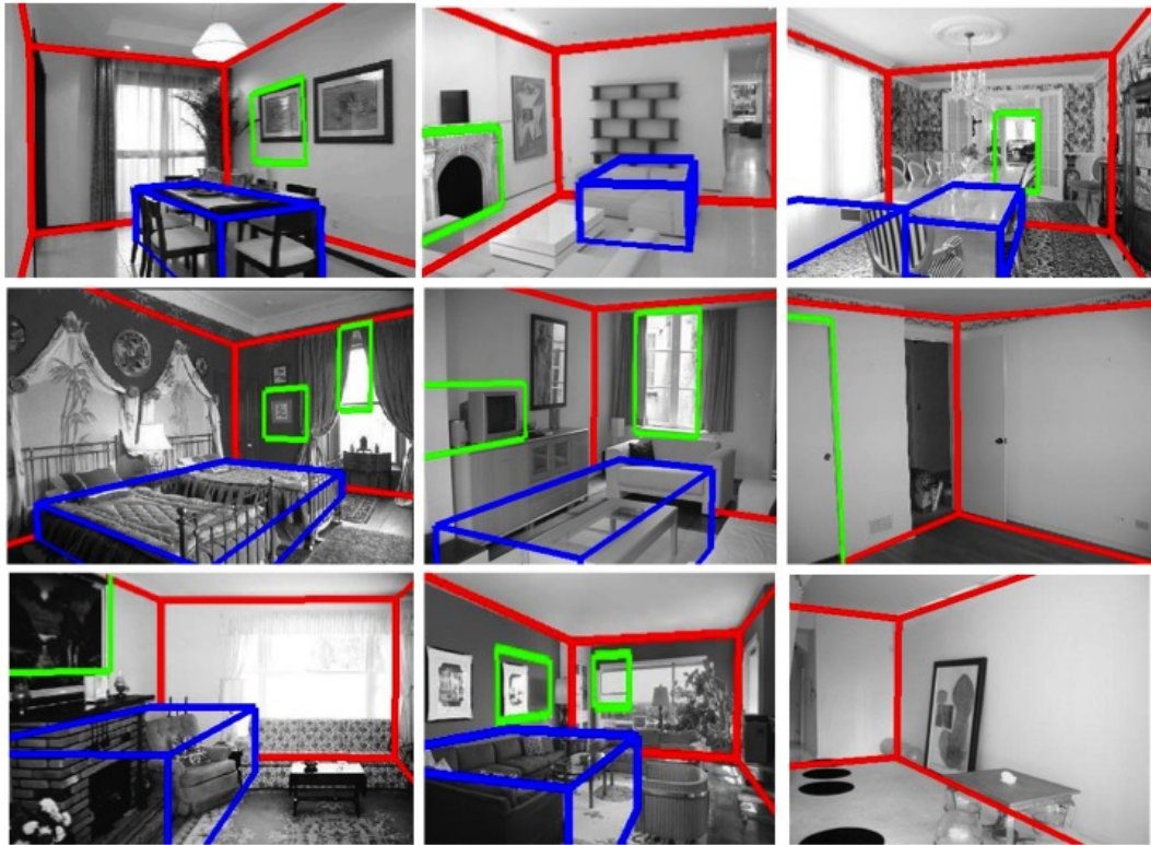
Figure 2.15: A few promising examples of full scene reconstructions estimated by our algorithm. We show in red the projection of the estimated room box, in blue the furniture objects, and in green the frames.
